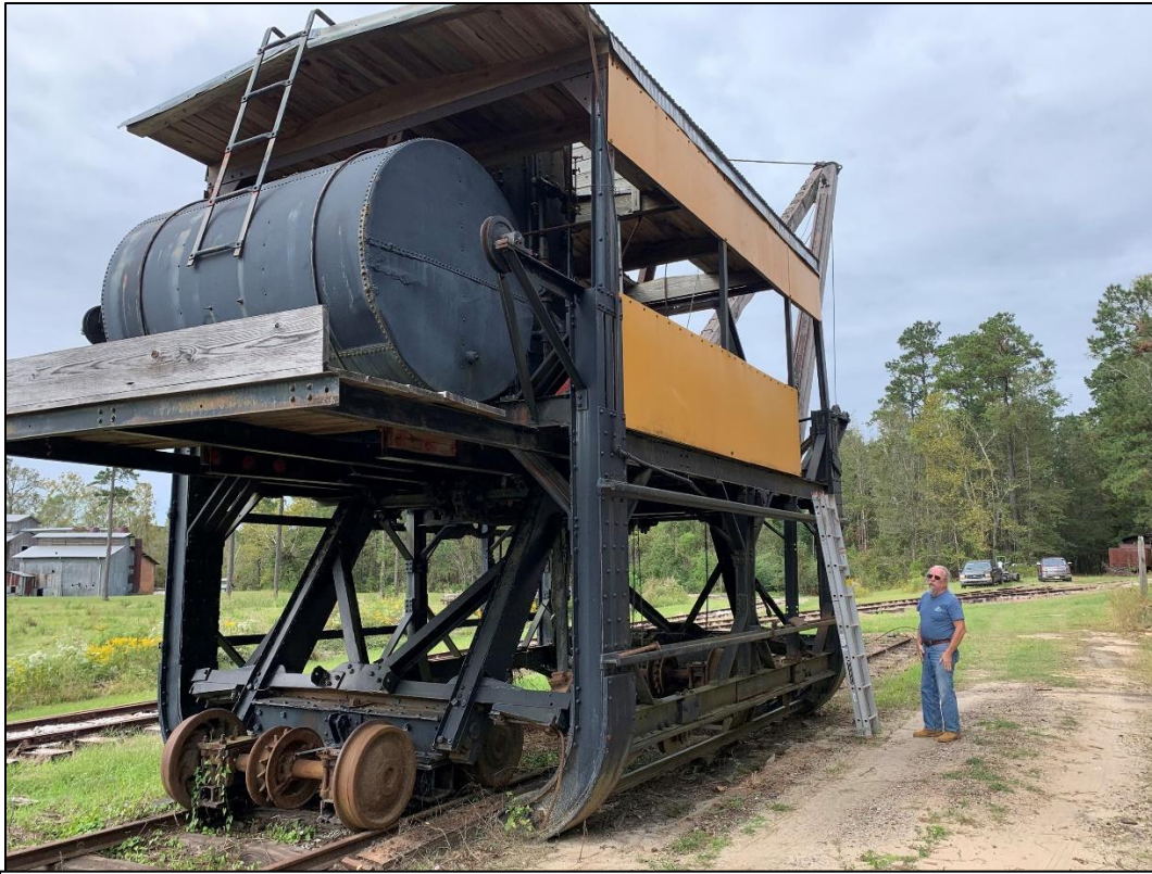
This is the Southern Forest Heritage Museum loader #1229 which has been restored for exhibition purposes—its boiler is not functional. Although the wheels are not raised, the loader's legs are down and resting on the long steel plates called shoes.
