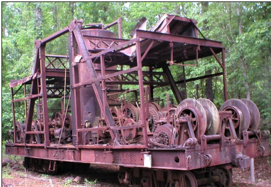
This Clyde skidder at the Southern Forest Heritage Museum is the only one known to exist. The booms that extended from both ends have been removed. It was a massive piece of equipment.
