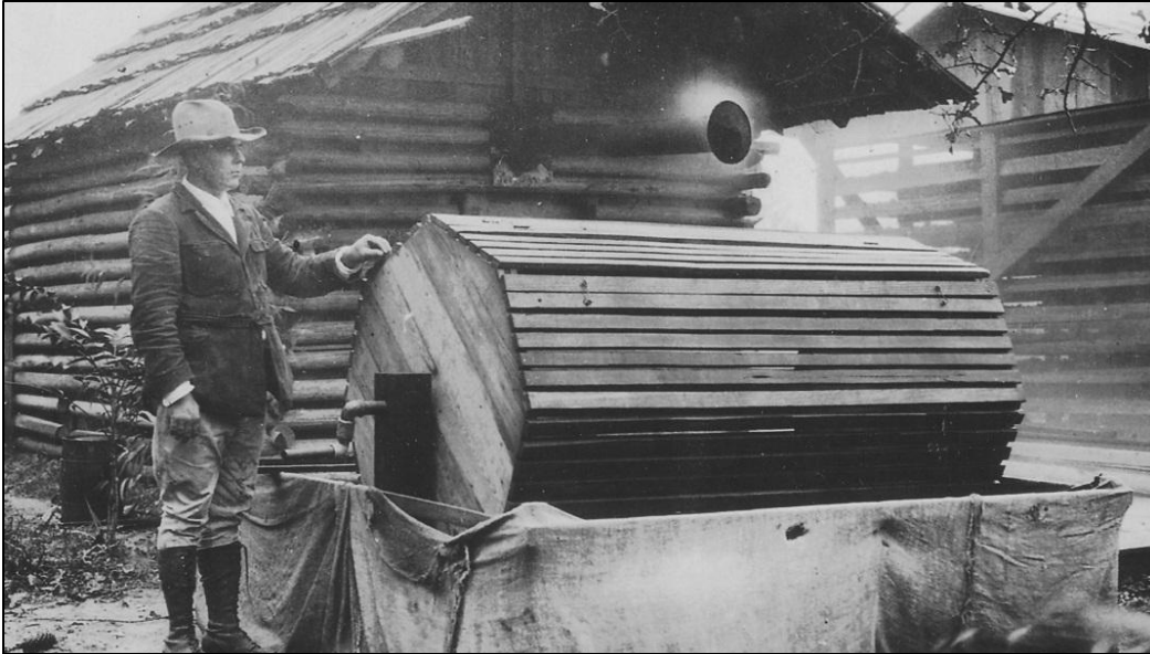
Luther Delaney inspecting a tumber built to separate seeds from pine cones. The cones were dried in the heated log cabin behind Luther. (Photo from Louisiana Office of Forestry)
