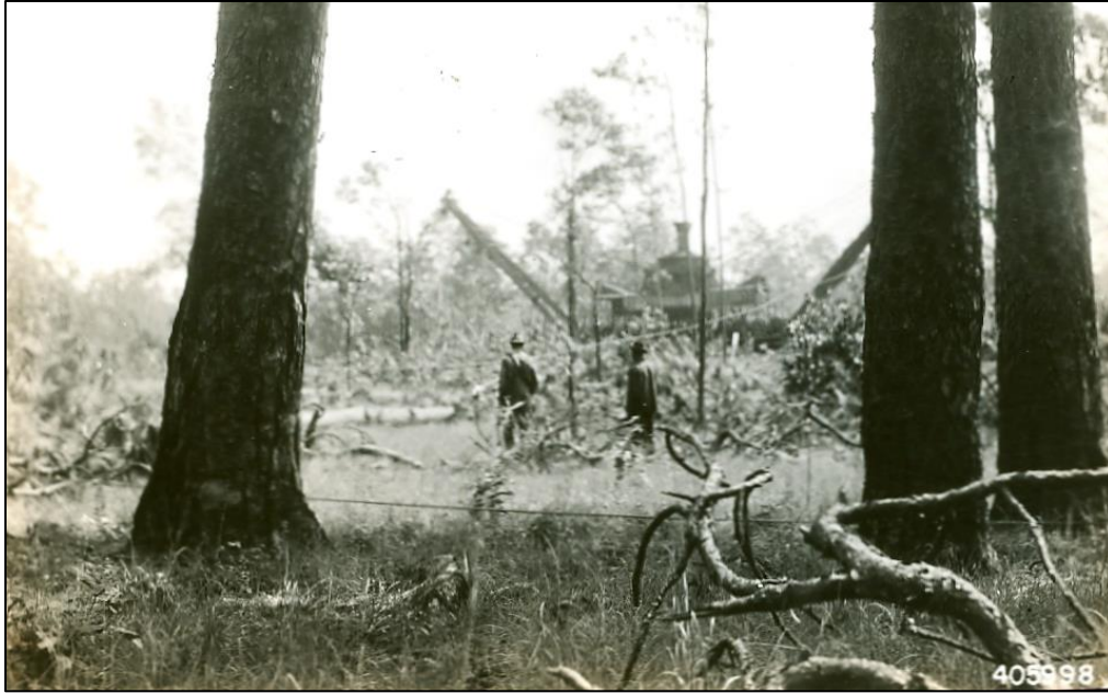
A close up of the skidder at work and the cabling involved. Notice the idler car stacked with chains, blocks, and tools. Meridian had three skidders at the time.
