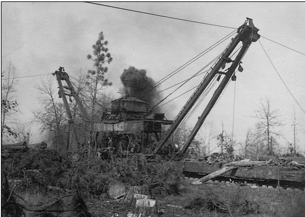
Taking in the scene from a distance, photographer Gerhart captured the entire skidder train at work. Meridian engine #303 pushes a series of log cars used as idlers and the skidder itself as it moves back into the cut over timber.
